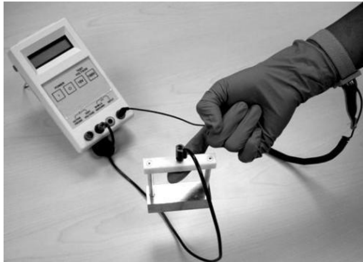
Figure 20: Test Wearing a Glove Using Constant Area and Force Electrode
