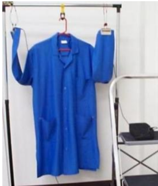
Figure 14: Alternate Point-To-Point Resistance Measurement
